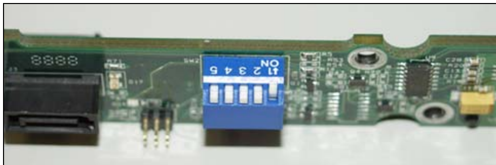
Figure 5 – Turn pin 1 to "ON" position
