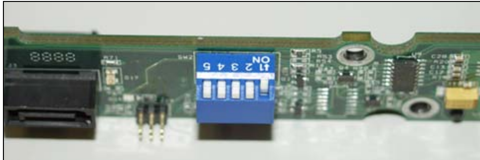
Figure 1 – Turn pin 1 to "ON" position
